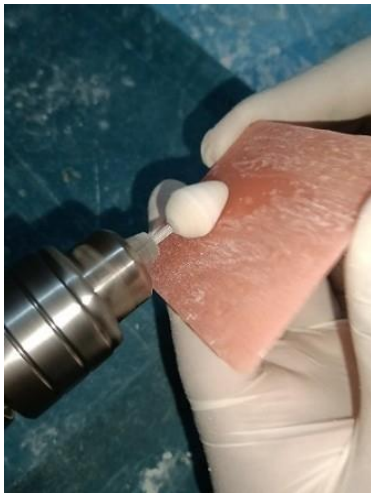
Figure 3. Polishing of Acrylic Resin Specimens
