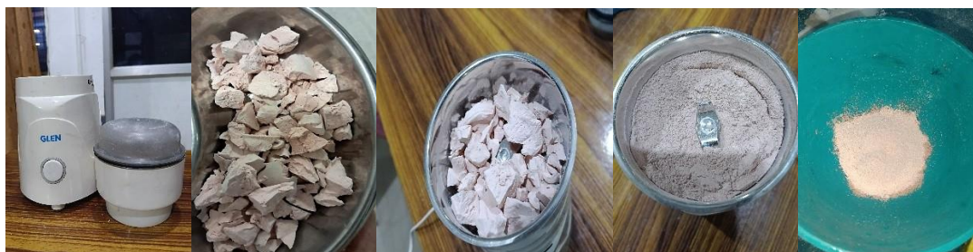
Figure 1. Fabrication of Alginate Polishing Powder
