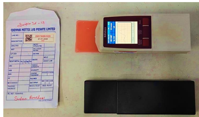
Figure 5. Surface Roughness Measurement Using Profilometer
