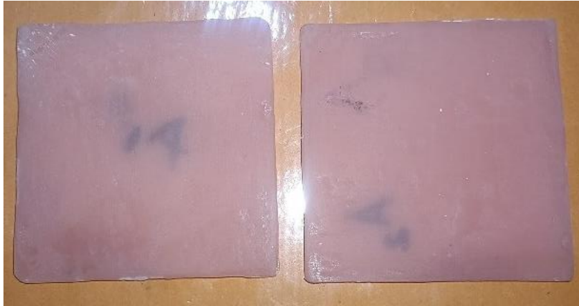
Figure 2. Fabrication of Acrylic Resin Specimens
