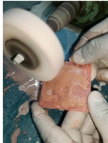
Figure 4. Buffing of Acrylic Resin Specimens
