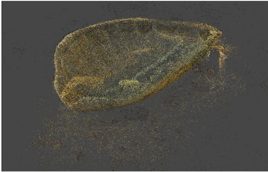
Figure 4. Dense point cloud generated from photogrammetric processing of a marine vertebrate remain within the Turtle Tomb cave system. The reconstruction shows high point density across the main structure, with surrounding noise attributed to suspended particles and low-light conditions during image acquisition.
